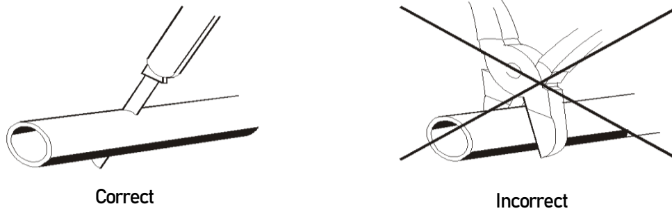
Fig. 16 – Cutting of the line before installation.
