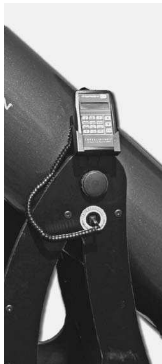
Figure 10.4 Digital setting circles are handy for finding objects that pose too difficult a challenge to locate by star-hopping. But, please, don't use them as an excuse not to learn how to star-hop.
