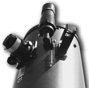
Figure 7.1 This amateur telescope has the best of both worlds: an 8 \times 50 straight-through finder as well as a Rigel QuikFinder unity finder. Note the 8 \times 50 ring mount's silver spring-loaded piston discussed in the text.
