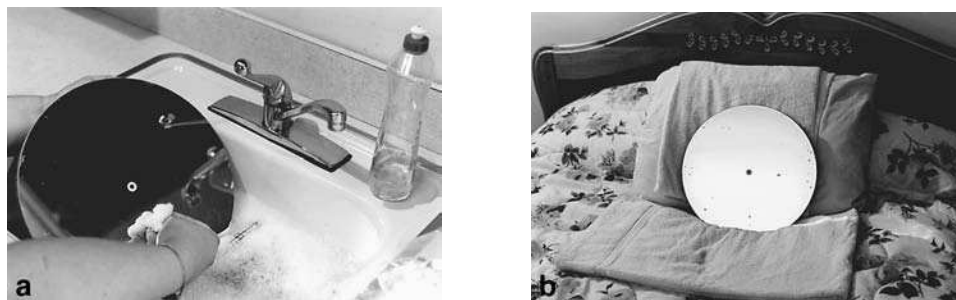
Figure 9.4 The proper way to clean a mirror: (a) after using compressed air or a camel-hair brush to remove any loose contaminants, wash the mirror in the sink using a gentle liquid dishwashing detergent and surgical cotton; (b) after rinsing the mirror with distilled water, tilt it nearly vertically to prevent water from puddling.
