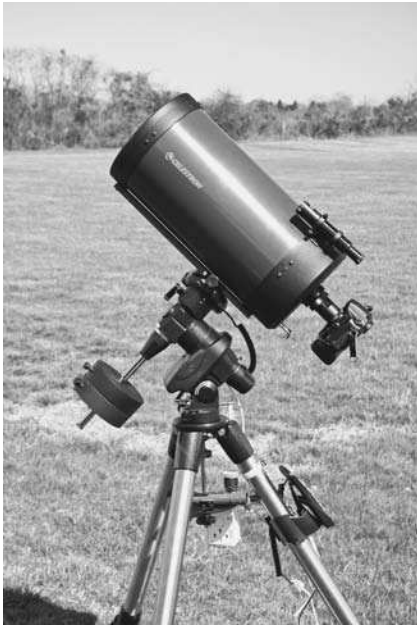
Figure 5.8 Celestron's C8-SGT couples its well-regarded 8-inch Schmidt-Cassegrain telescope with the Advanced Series CG-5 German equatorial mount.
