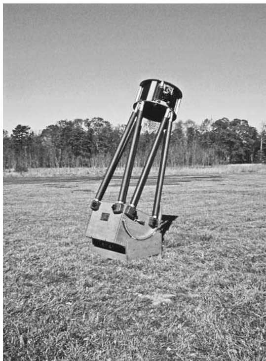
Figure 5.5 The Obsession 15, an outstanding 15-inch f/4.5 Newtonian reflector comes on a state-of-the-art Dobsonian-style alt-azimuth mounting.
