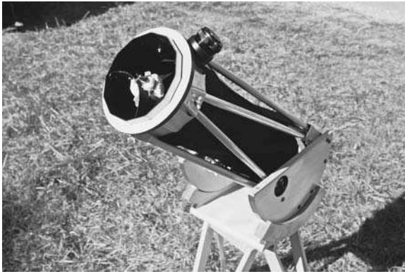
Figure 5.7 The 6-inch f/5 Stargazer Steve Truss Tube Kit 6 can be easily disassembled for compact storage, making it a perfect traveling companion by land, sea, or air.
