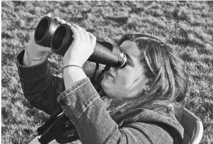
Figure 4.4 The author's daughter, Helen, viewing through a pair of Fujinon 16 \times 70 FMT-SX binoculars. Note how she is supporting the ends of barrels, rather than gripping them around their prisms. Although still a tiring exercise, this is the best way to support giant binoculars by hand.
