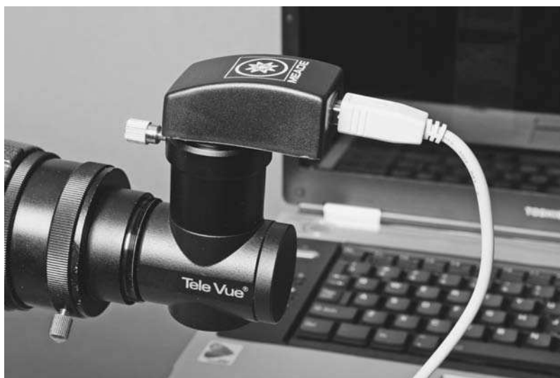
Figure 7.7 The Meade Lunar Planetary Imager (LPI) is one of the smallest, lightest digital astro-imagers sold today. Photo by Brian Kennedy.
