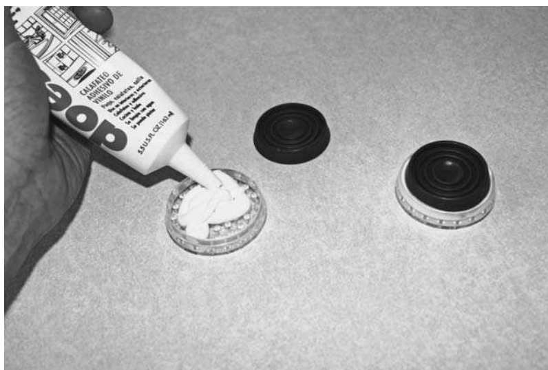
Figure 8.10 Jim Dixon's homemade vibration suppression pads.
