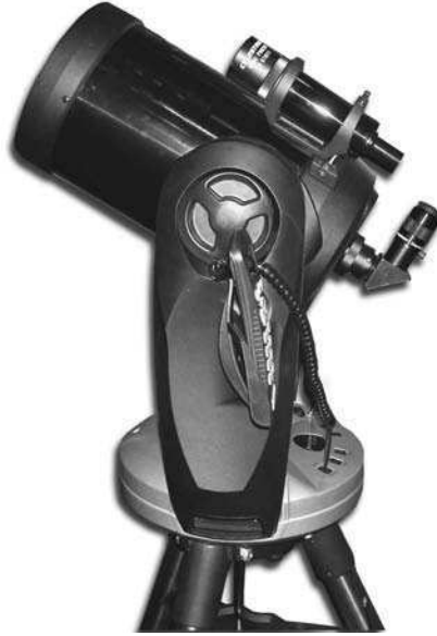
Figure 3.5 Schmidt-Cassegrain telescopes, like the Celestron CPC shown here, remain very popular among today's amateur astronomers. Photo by Kevin Dixon.
