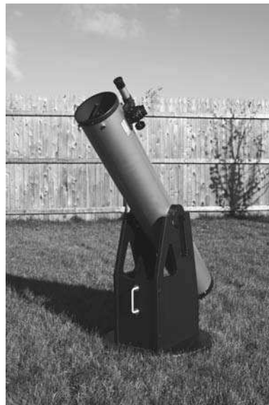
Figure 3.3 This 6-inch f/8 Newtonian reflector on a basic Dobsonian mount would be an ideal first instrument for any new stargazer.
