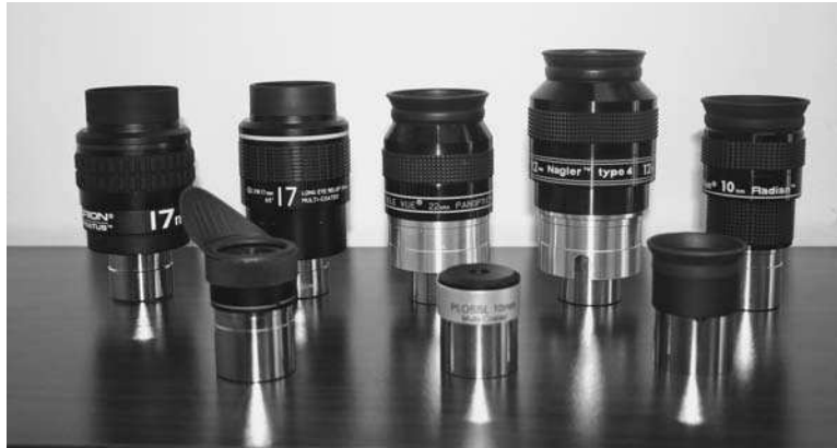
Figure 6.1 A selection of eyepieces. Left to right in the back row: Orion 17-mm Stratus, Vixen 17-mm Lanthanum LW, Tele Vue 22-mm Panoptic, Tele Vue 12-mm Nagler Type 4, and Tele Vue 10-mm Radian. Eyepieces in the front row include, from left to right, the 9-mm HD orthoscopic, a generic 10-mm Plössl, and a no-name 12-mm Kellner.
