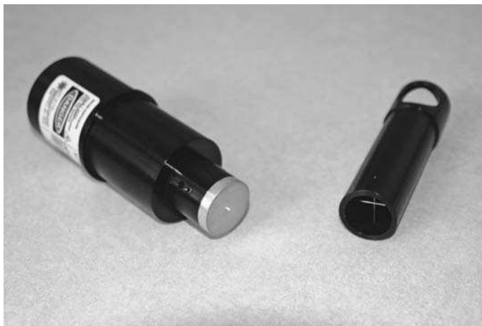
Figure 7.5 Two tools for checking telescope collimation: a laser collimator (left) and a combination sight tube/Cheshire eyepiece (right).
