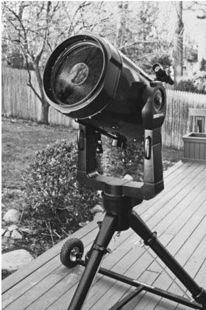
Figure 5.10 Meade's RCX400 is a state-of-the-art virtual Ritchey-Chrétien telescope thanks to the front corrector plate's influence on entering starlight before it strikes the spherical primary mirror and hyperbolic secondary mirror.
