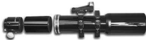
Figure 5.2 The Stellarvue SV80D includes an innovative split tube. Keep the short center section in place for traditional viewing with one eyepiece and a star diagonal or remove it when using a binocular viewer. Photo courtesy of Stellarvue Telescopes.
